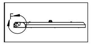
OPTIONAL: The angle of the fixture can be changed by utilizing a combination of mounting the gussets in reverse as shown, and the different mtg. screw locations on the fixture. Available angles: 0°, 20°, 45°. FIXTURE MUST BE MOUNTED IN 0° POSITION TO BE DARK SKY COMPLIANT.
