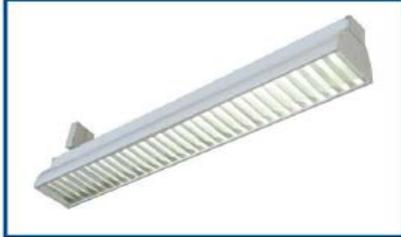
A direct/indirect lighting fixture that makes a bold statement, complementing design elements such as stone, metal, brick and glass. Industrial look provides a modern aesthetic. Available with slots in reflector for indirect light or solid reflector. Available standard in galvanized steel finish or powder coated black. Mounts with cable kit. Louver is matte silver anodized parabolic.
