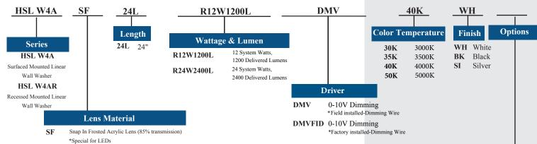
Example: HSL W4ASF24LR12W1200LDMV40KWH
